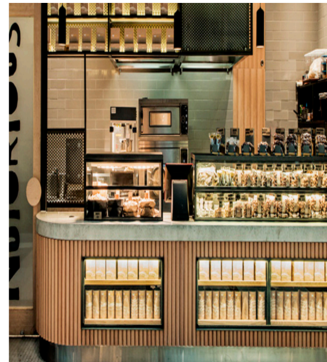
Above -Profile 683- 1.5" wide half round by 3/4" thick! - White Oak
